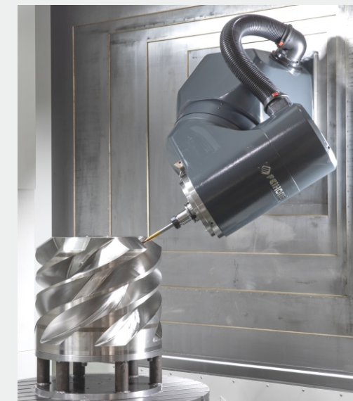
Helical rotor processing
