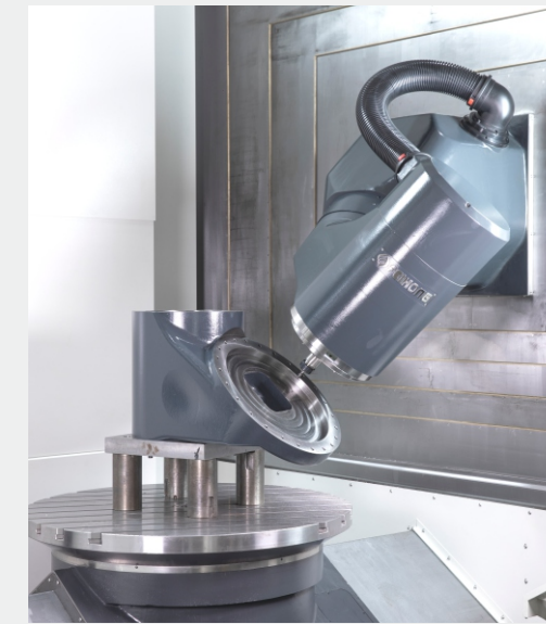
45° inclined surface processing
